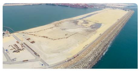
The entirety of the dredging works for both phases at WCT-1 is near complete.
